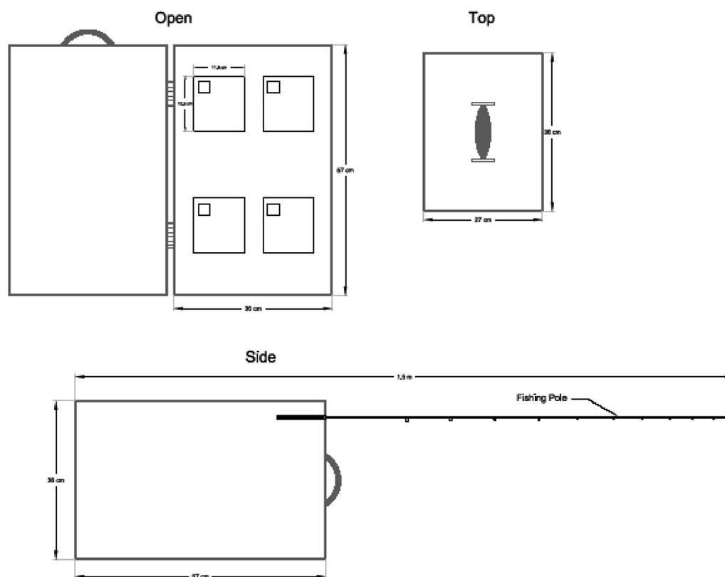
**Fig. 1.** Four SKC Model 224-PCXR8 Personal or Area Air Sampling Pumps were attached with heavy duty Velcro inside a 60 cm (diagonal length) hard side upright suitcase. Holes were drilled to accommodate sampling in three directions at 45 cm and an extendable fishing pole (Master, Model GC850) was attached to the back of the suitcase to accommodate sampling at 1.5 m.
