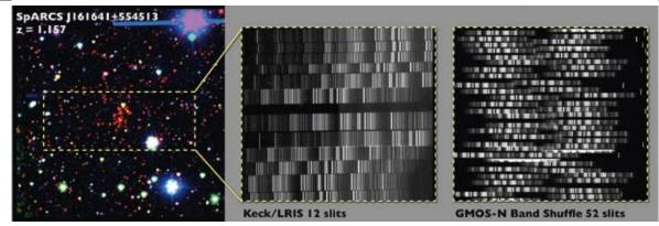
In band-shuffle mode, the entire central region of the chip is shuffled to the top or bottom of the chip, which means no space is required between slits. While it is technically less efficient in the total use of the GMOS chips (only one third of the area is used, whereas up to half can be used with micro-shuffle), it is perfect for high-z clusters. With a band-limiting filter we can now typically place 35 - 55 slits within an area of about  $3.0 \times 1.7$  arcminutes around these clusters.
