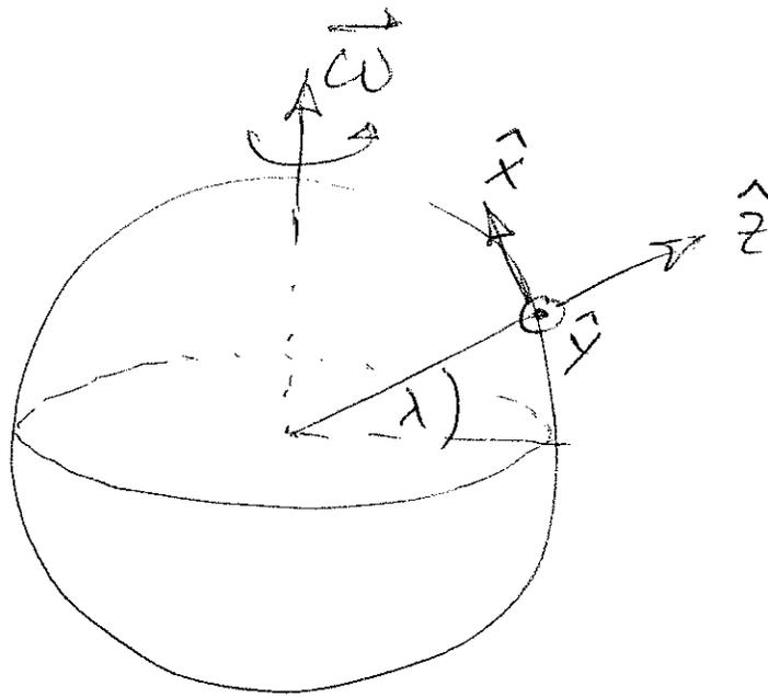
Q : Shown is the frame one would use for a pendulum in the ~~the~~ northern hemisphere. How do we know the direction of  $\vec{\omega}$  is correct?
