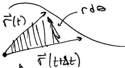
$$dA = \frac{1}{2} r^2 d\theta \Rightarrow \frac{dA}{dt} = \frac{1}{2} r^2 \frac{d\theta}{dt} = \frac{1}{2} r^2 \dot{\theta} = \frac{l}{2\mu} = \text{const.}$$
