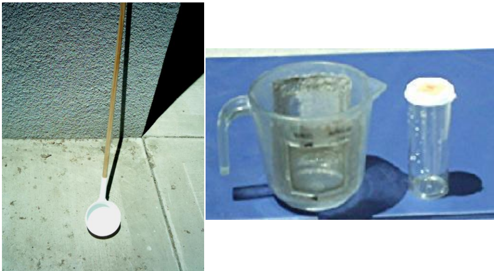
Figure 1. Picture of a dipper, a concentrator cup, and a snap-cap vial. Photos by M. R. Sanford.
