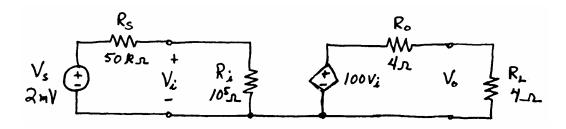
$$A_{i} = \frac{V_{o}}{V_{i}} = A_{oc} \frac{R_{L}}{R_{o} + R_{L}} = 100 \frac{4}{4 + 4} = 50$$
