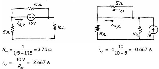
Then the total current due to both sources is  $\emph{i}_{s}=\emph{i}_{s,v}+\emph{i}_{s,c}=-3.333\,\textrm{A}$  .
