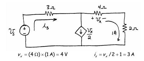
Applying KVL around the outside of the circuit:
