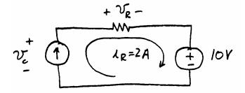
As shown above, the 2 A current circulates clockwise through all three elements in the circuit. Applying KVL, we have
