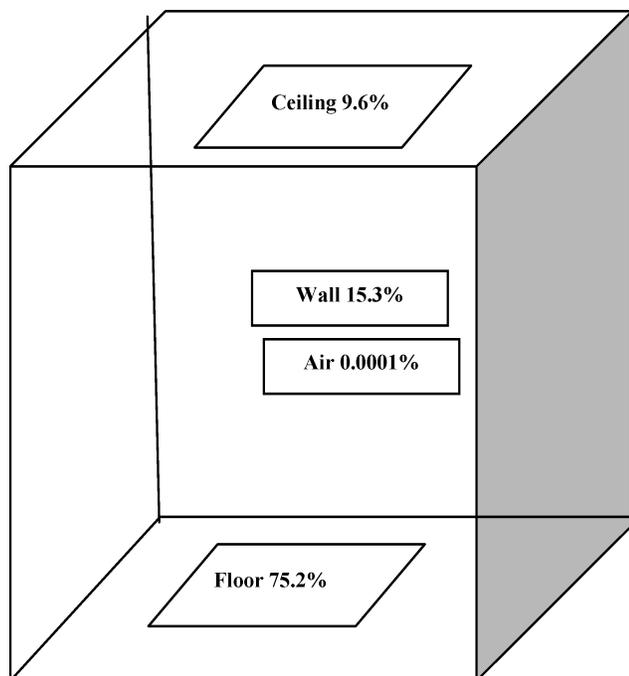
**Fig. 2.** Cypermethrin was applied using a Raid Deep Reach Fogger in a 3 m × 3 m × 3 m carpeted test room. Surface residue (SR) was measured using foil coupons and 75% of cypermethrin applied was accounted for. Air was monitored using Aircheck Samplers and XAD-2 tubes.
