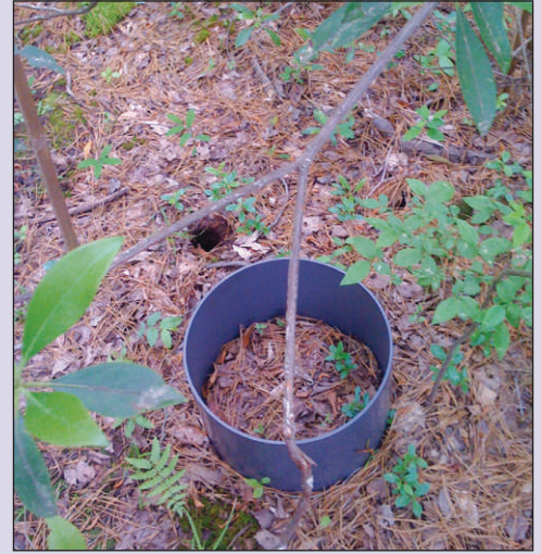
Figure 4. Soil collar for in situ methane quantification.
