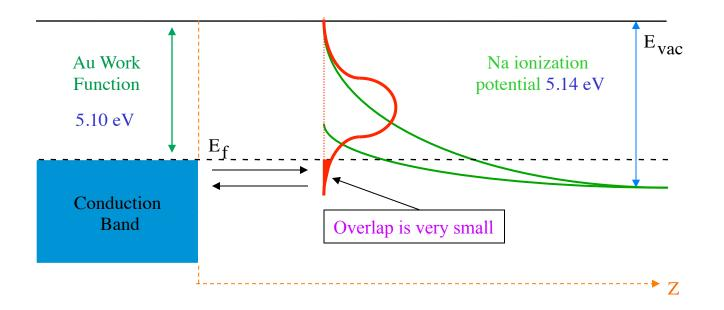
• For Au metal, or a bulk-like film, the overlap between the conduction band and the Na *s* level is small, leading to a neutral fraction of  $\sim 2\%$
