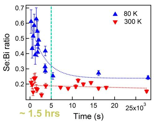
Time dependence of Se:Bi ratio at an altitude angle  $\varphi$ =0° and an azimuth angle  $\phi$ = 12.5°
