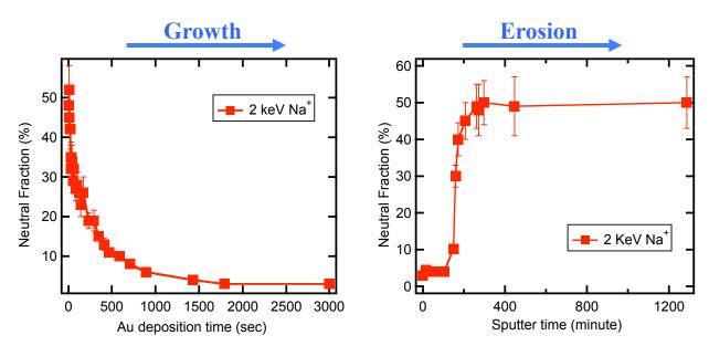
• The erosion and surface diffusion of Au due to ion bombardment forms nanoclusters.
