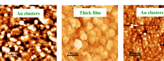
Au nanocrystals formed by sputtering with Ar<sup>+</sup> ions
